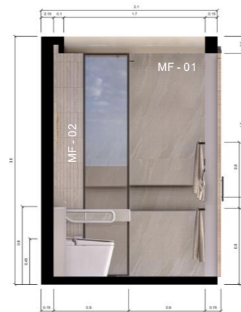
Interior Elevation D
