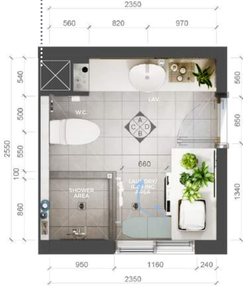
Bathroom Floor Plan Floor Area = 5.99 sqm (approx 6.0 sqm)
